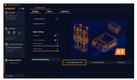
Your haptic system should start moving and vibrate following a factory haptic pattern.
