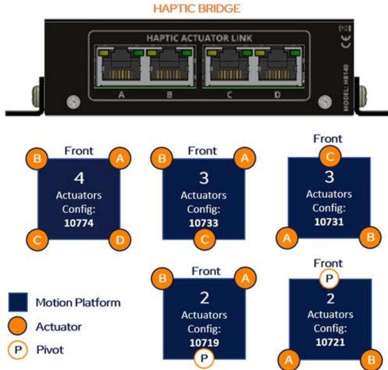
Make sure to connect each actuator (RJ45) cable to the lettered port of the Haptic Bridge as indicated in the image above.
