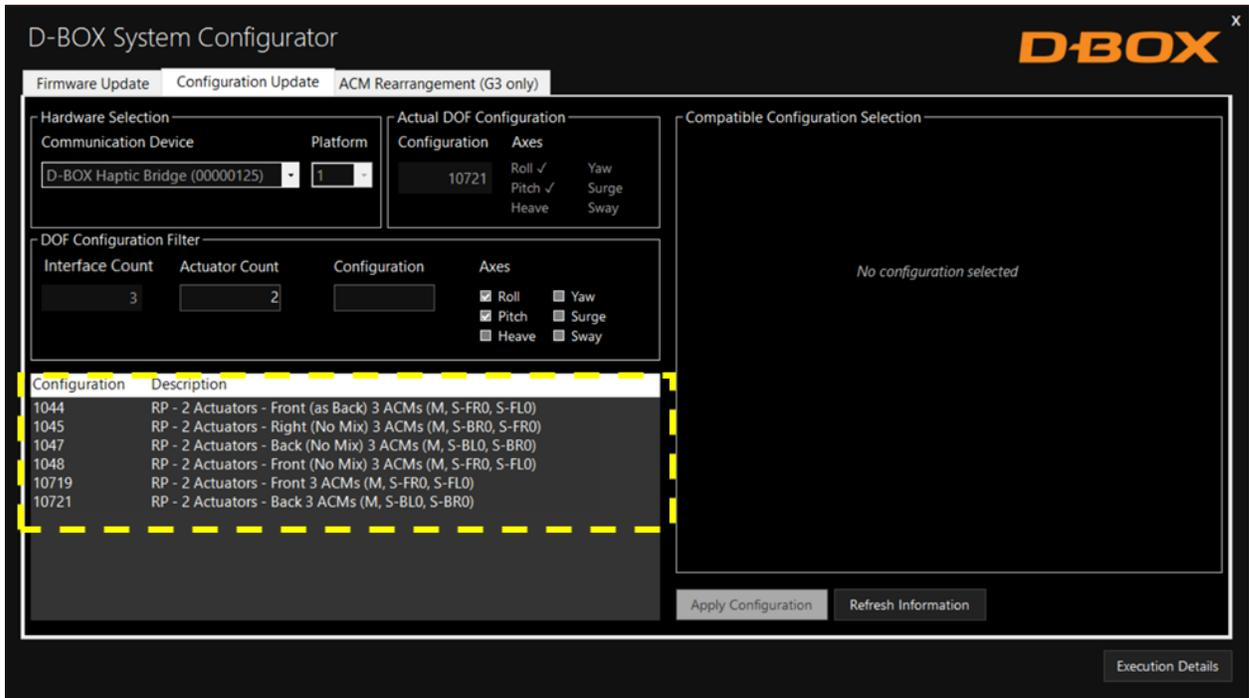
By selecting a configuration, its layout appears in the Compatible Configuration Selection box. The layout displays the positions of the Haptic Actuator(s) on the simulator, chair, or platform, and the associated port on the Haptic Bridge.
